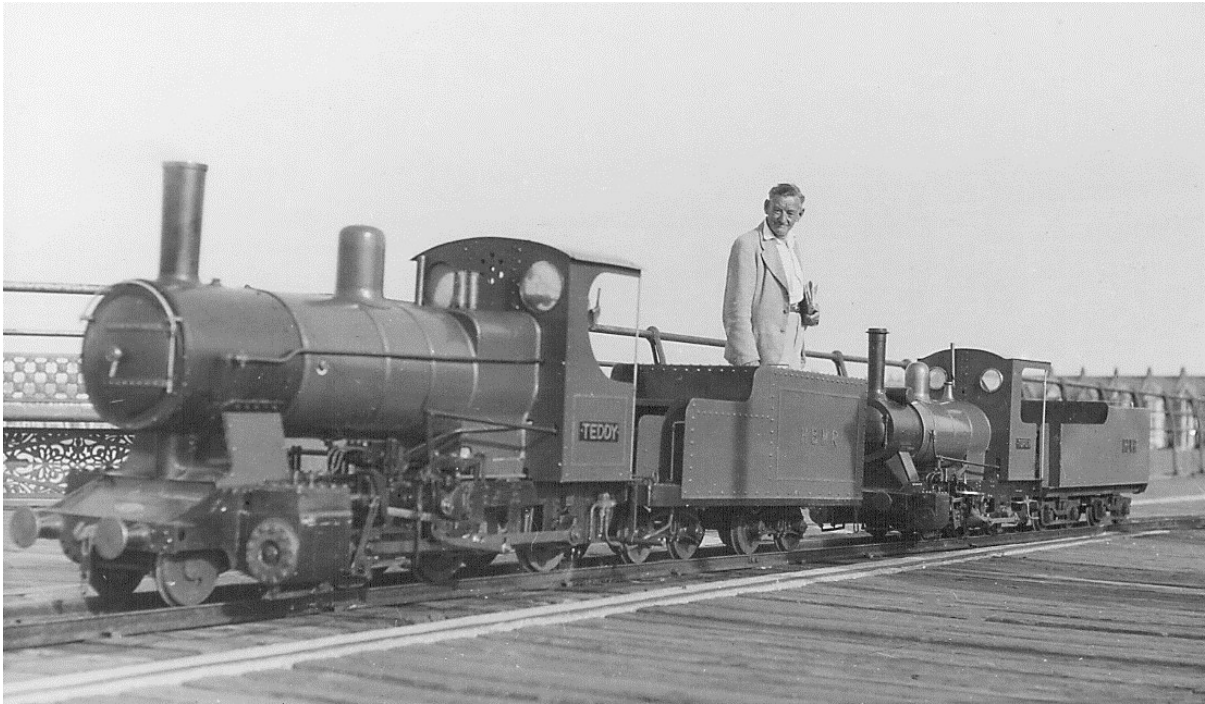
A nice view of 2-6-0 "Teddy" and 0-6-0 "Topsy" together at the S bend just north of the station, allowing a comparison between them. Both locomotives had bogie tenders. ( Tower Studio Postcard 1950. M. Easdown/Marlinova Collection )
